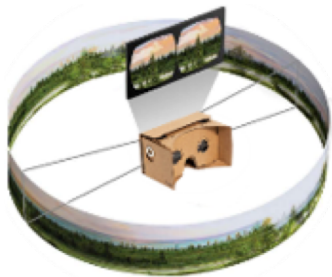
Figure 2: Stereoscopic effect and virtual environment perception on Google Cardboard.
