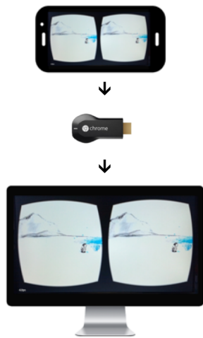
Figure 1: View on smartphone and secondary screen by mirroring with Google Chromecast over Wi-Fi.
