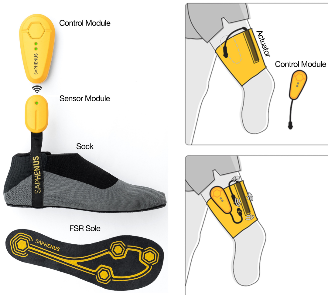
Figure 1: The Suralis ® system, developed by Saphenus Medical Technology GmbH in Vienna, Austria, is designed to measure ground-contact pressure using force-sensitive resistors (FSRs) located in four areas of a sock. The data collected by the sensor module transmits to a control module, which connects to four vibration motors.
