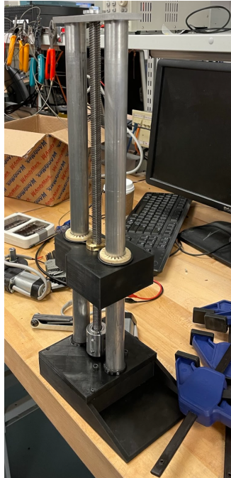
Figure 5. Initial plastic prototype had high mechanical play and high current draw
