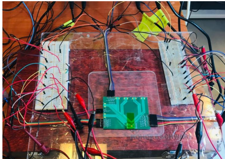
Figure 20: Radar IC Biasing Circuitry
